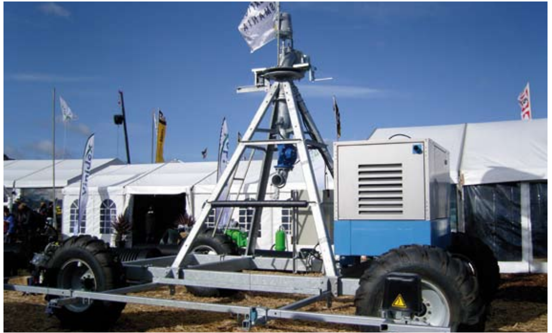
A centerliner irrigator
